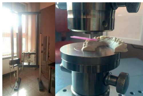
Fig. 1. The testing machine Zwick Roell Z020 with the model of the dentition
