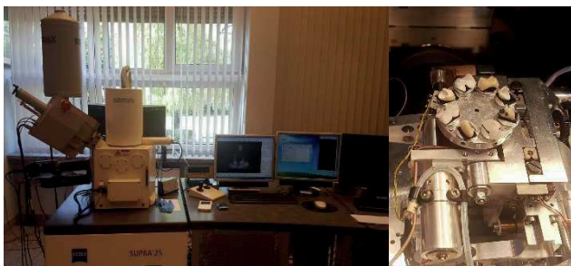
Fig. 3. Scanning electron microscope and the sample mounted on a stand in the chamber of the microscope
