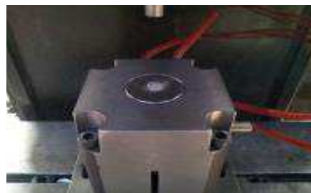
Fig. 1. The mould used in the pressing of the powder
