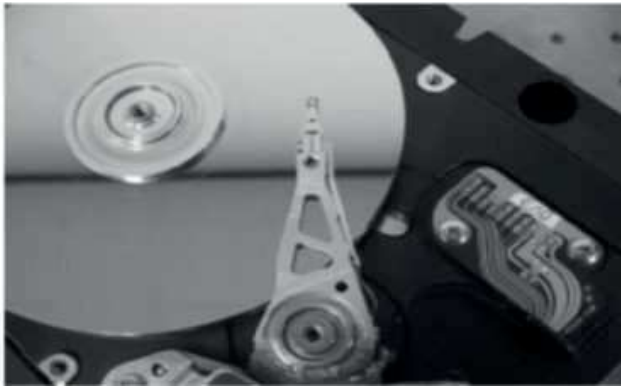
Fig. 2. Compound actuator with PZT MA used for vibration sensing
