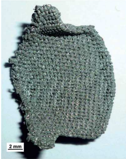
Fig. 6. Scaffold produced in SLM process; bottom view
