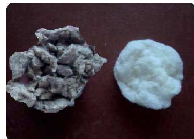
Fig. 3. Produced pulp (left) and alpha-cellulose (right) from Turkish pine sapwoods
