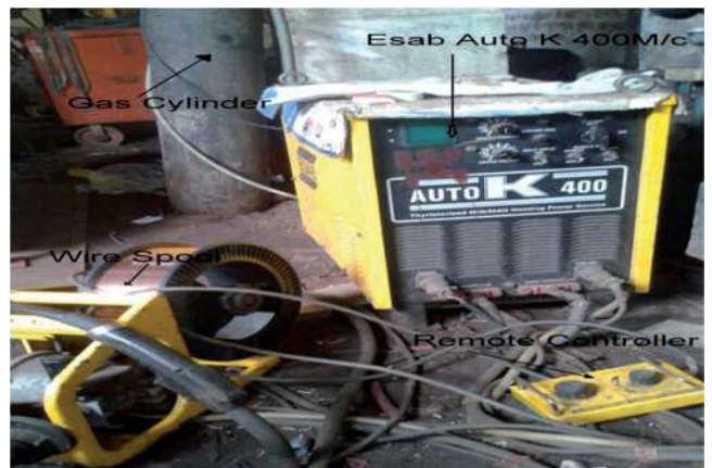
Fig. 1. Photographic view of welding set-u
