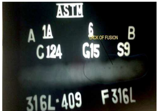
Fig. 5. Copies of X-ray radiographic film for sample no. 8
