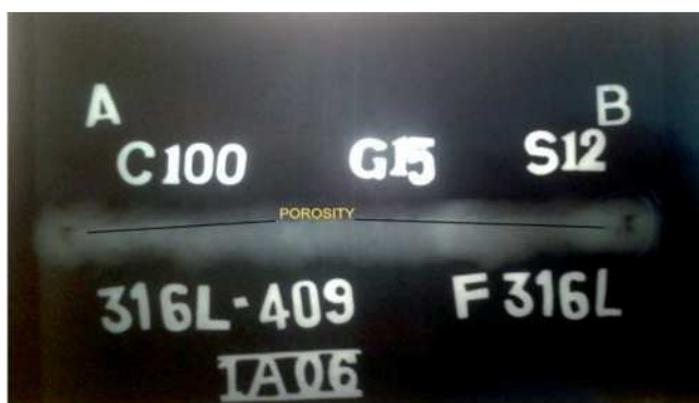
Fig. 9. Copies of X-ray radiographic film for sample no. 2
