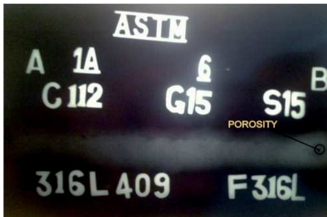
Fig. 7. Copies of X-ray radiographic film for sample no. 5
