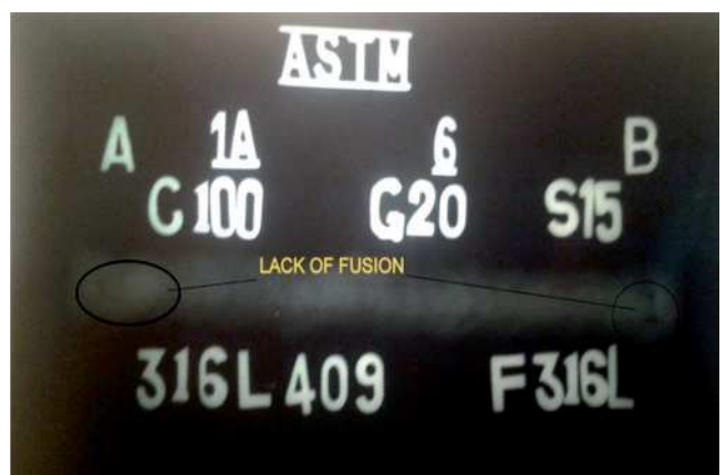
Fig. 6. Copies of X-ray radiographic film for sample no. 3
