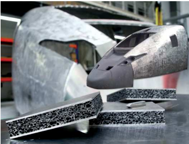
Fig. 1. An exemplary application of composite materials based on aluminium metallic foams in the construction of a locomotive prototype for high-speed rail [6]
