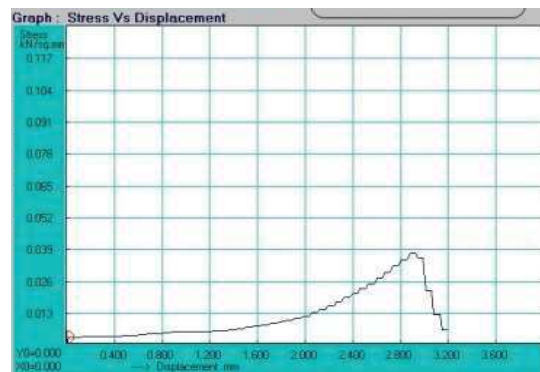
Fig. 9. Stress vs. displacement of sample without FSW treatment
