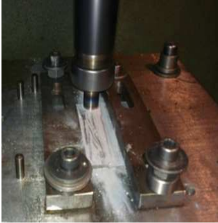
Fig. 4. Stir welding process with Zn powder
