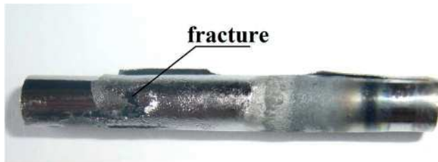
Fig. 5. The way the hollow cathode looks at a vacuum level P=5 \cdot 10^0 Pa (Experiment 7)
