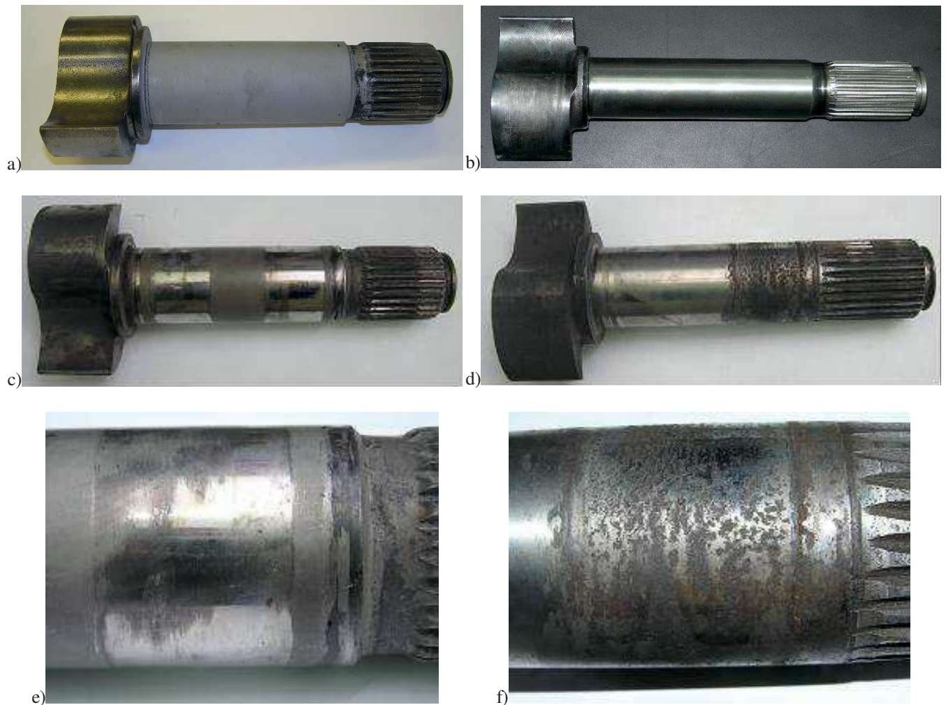
Fig. 2. Macroscopic images of the expander regenerated with multiplex technology (left column) and original one (right column): a),b) – expanders before installation in the bus, c),d) – expanders after 9 months of operation, e),f) – enlargement of the working surface located at the splines
