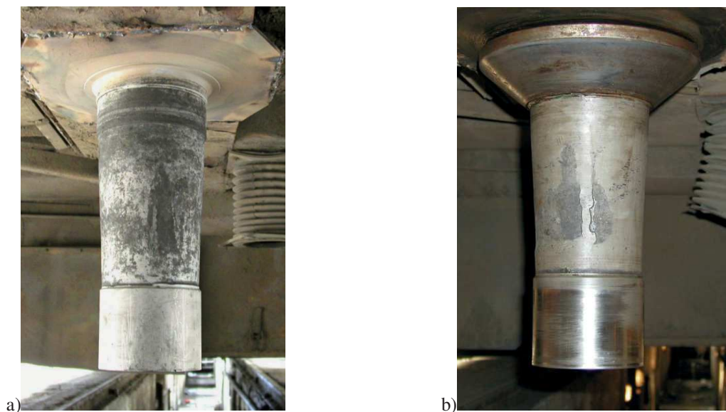
Fig. 7. The pintle view: a) the pintle prepared for tests b) the pintle after regeneration tests
