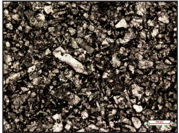
Fig. 3. The surface of the obtained samples with the reinforcement fraction of 20-50 μm
