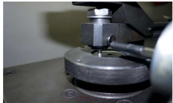
Fig. 1. T-01 tribological tester used for the studies
