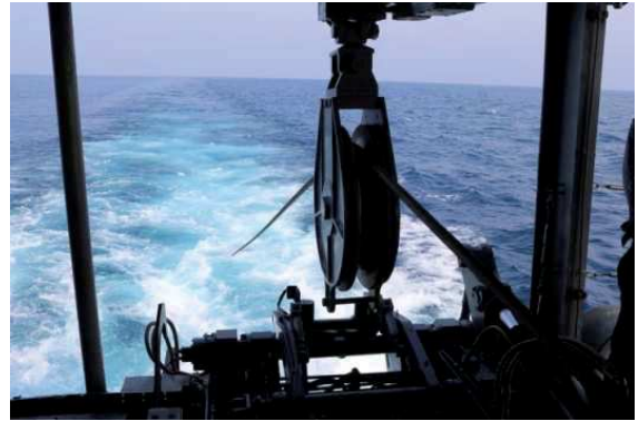
Fig. 7. Sheave based handling system
