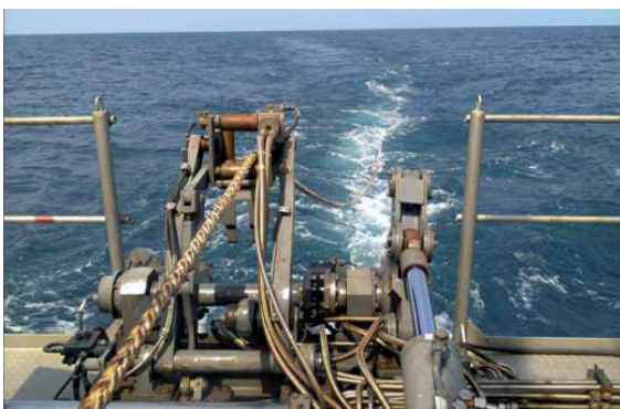
Fig. 6. Roller based handling system
